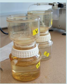
A filtration system captures organic material in water samples.
