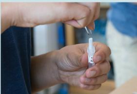
Filters are carefully folded and placed in vials.
