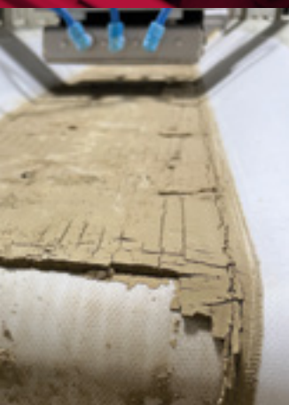
Above: A vacuum belt filter at the site of Alithic, a UW spin-off company (based on technology developed by Anex and Wang) that captures carbon and stores it in a concrete replacement.
